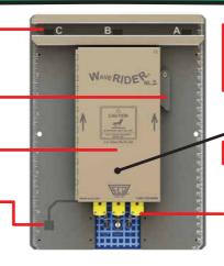
**Extractor handle:** This disconnects the M.O.L.E.® Profiler from the connector
