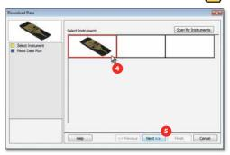
6. Select the desired data run and then click the Finish command button to complete the wizard and read the data run from the M.O.L.E.® Profiler. When the data run has been downloaded, the software will prompt the user to name and save the data run file (\*.XMG).
